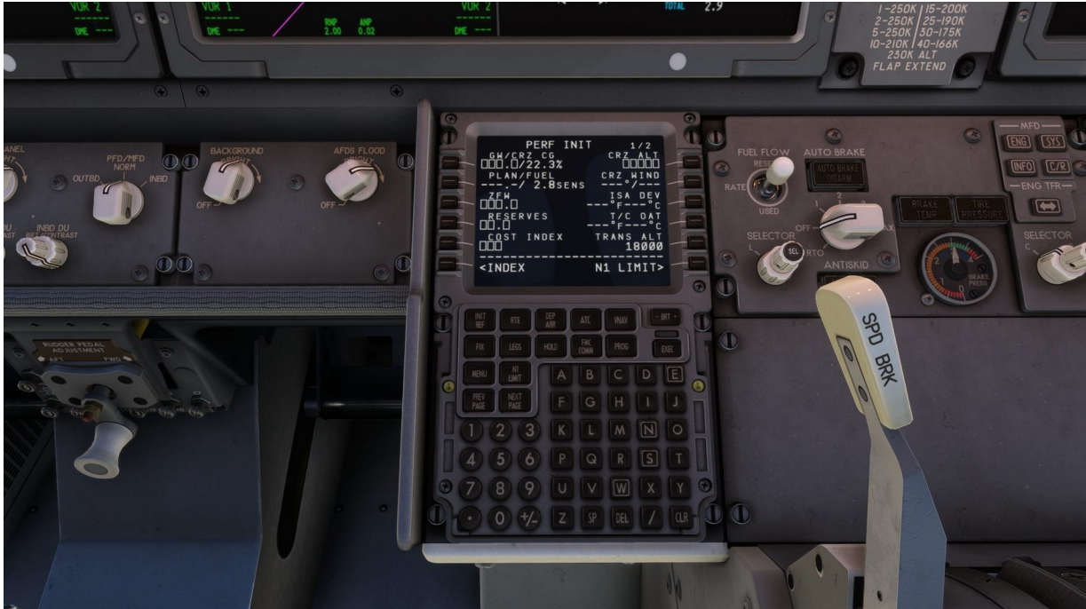
Figure 3: CDU on the PERF-INIT page; Autobrake and Speedbrake to the right of it
